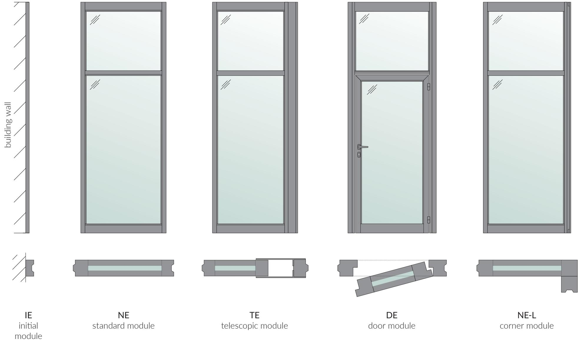
Standard modules of the Optimal 110 / Optimal 110 plus systems
